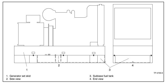
Figure 6-2 Subbase Fuel Tank
